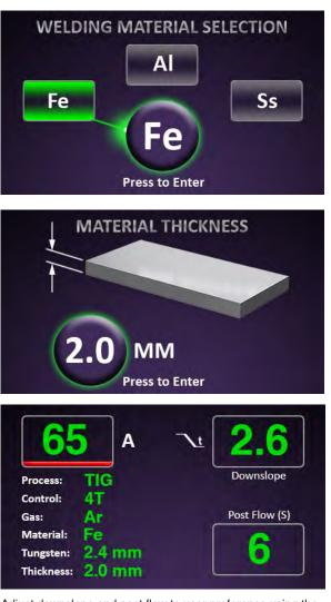
Adjust downslope and post flow to user preference using the knobs on the right of the screen.
