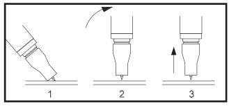
At the end of the weld release the trigger and allow the power and gas to switch off before moving the torch from the weld.
