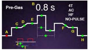
9) Press the control knob to select the parameter. The red LED will now flash. Adjust the value by rotating the control knob. This can be adjusted from 0.1 to 0.3 seconds. The value is displayed on the digital display (B) Press the control knob again to accept the setting.
