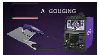
Hold the torch so that the nozzle is 1-2mm from the workpiece before starting the torch. Angle the torch 40 Deg. to the workpiece with a small gap between the torch tip and the workpiece. Maintain an approximate 40 Deg. angle to the workpiece as you move along the gouge in the direction of the uncut material. Keep a small distance between the torch tip and the molten metal to avoid reducing consumable life or damaging the torch.
