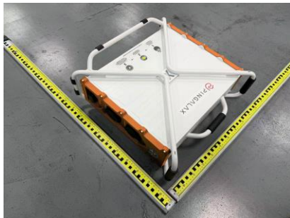
Battery/电池 (PHS3600P-UK-B 72V*8 4Ah*8 2304Wh)
