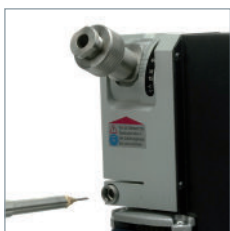
Precise adjustment of the electrode's stick-out.
