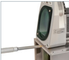
Precise adjustment of the electrode's stick-out.
