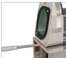
Precise adjustment of the electrode's stick-out.
